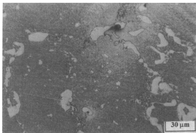
Fig. 3 Optical micrographs of used roller material. (a) Unswelled portion. (b) Swelled portion
